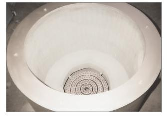
$4^{1}/2$ " of firebrick insulation and four-ring cast iron burner for heating a model 175 high temperature melting furnace.
