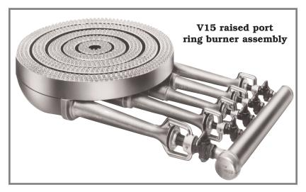
The *Buzzer* raised port ring burner is the Clydesdale workhorse of our industrial ring burner family. They are ideal for use in high ambient temperatures where resistance to radiated heat is required. Each ring is constructed of cast iron to provide exceptional strength and ruggedness, making them dependable performers in the metal working industries, heat treating, tool room, and foundry.
