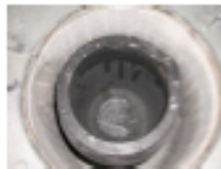
Crucible in melting furnace
