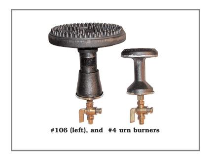
and combustion space. They also have a slotted head design which allows secondary air to pass through the center, producing shorter, more efficient and uniform flames. These models can be fitted with extension nipples to raise the burner head closer to the item being heated. This will take advantage of better efficiency and better heat transfer.
